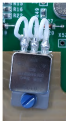
(b) TO 封装器件引出线应力释放
