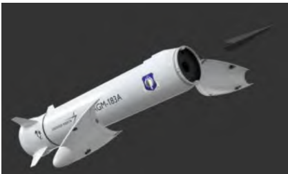
(b) AGM-183A 头体分离 (b) Separation of AGM-183A's body and head
