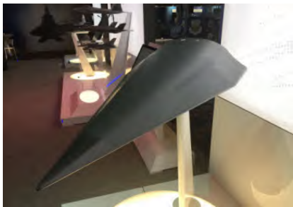
(a) AGM-183A 头部乘波体 (a) Wave-rider of AGM-183A's head
