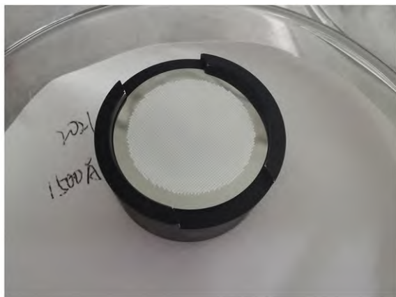
图6 具有栅网支撑的Al滤光片样品 Fig. 6 Al filter sample with mesh supported
