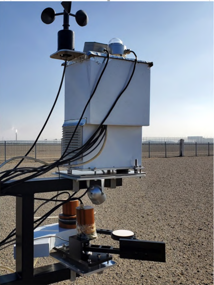
(b) 局部(白板位于测量光路中) (b) Partial (white plate is located in the measuring optical path)
