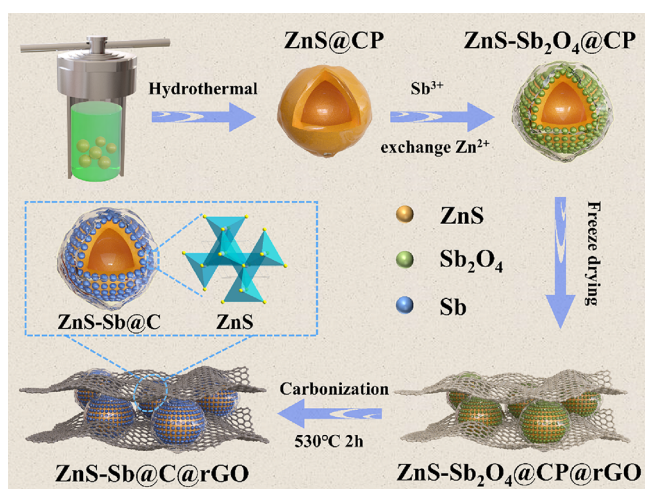
Figure 1. Schematic diagram of the ZnS-Sb@C@rGO composite.
