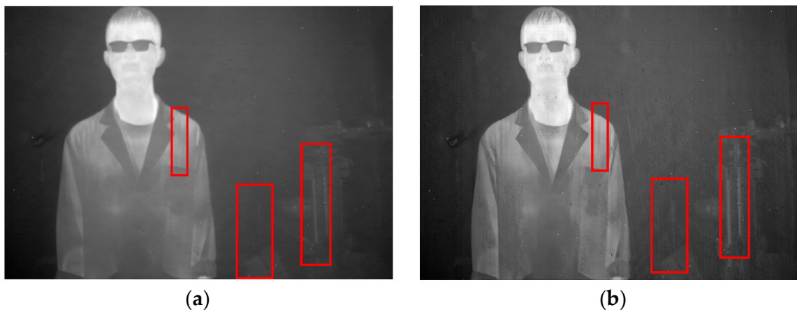
Figure 12. Denoising effects of ablation experiment on an image of a person: (a) Non-MIDILatLRR; (b) proposed method.
