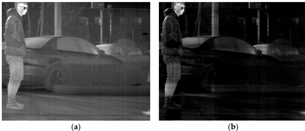
Figure 9. Adaptive decomposition result image: (a) Original image; (b) DS_n Extracted by MIDILatLRR.
