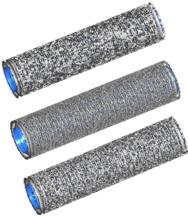
Fig. 7 Distribution of vortex core in needle
