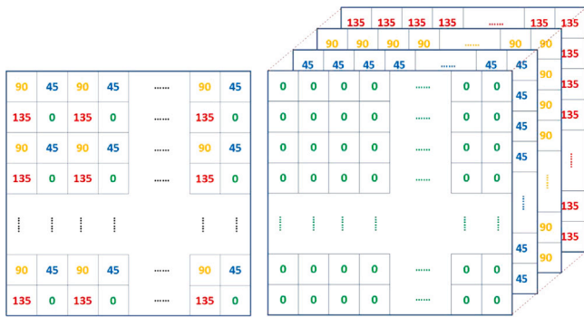
Fig. 5. Schematic of polarization SR data restoration. The left image shows the original measurement data from a DoFP; the right image shows the data after polarization SR reconstruction.
