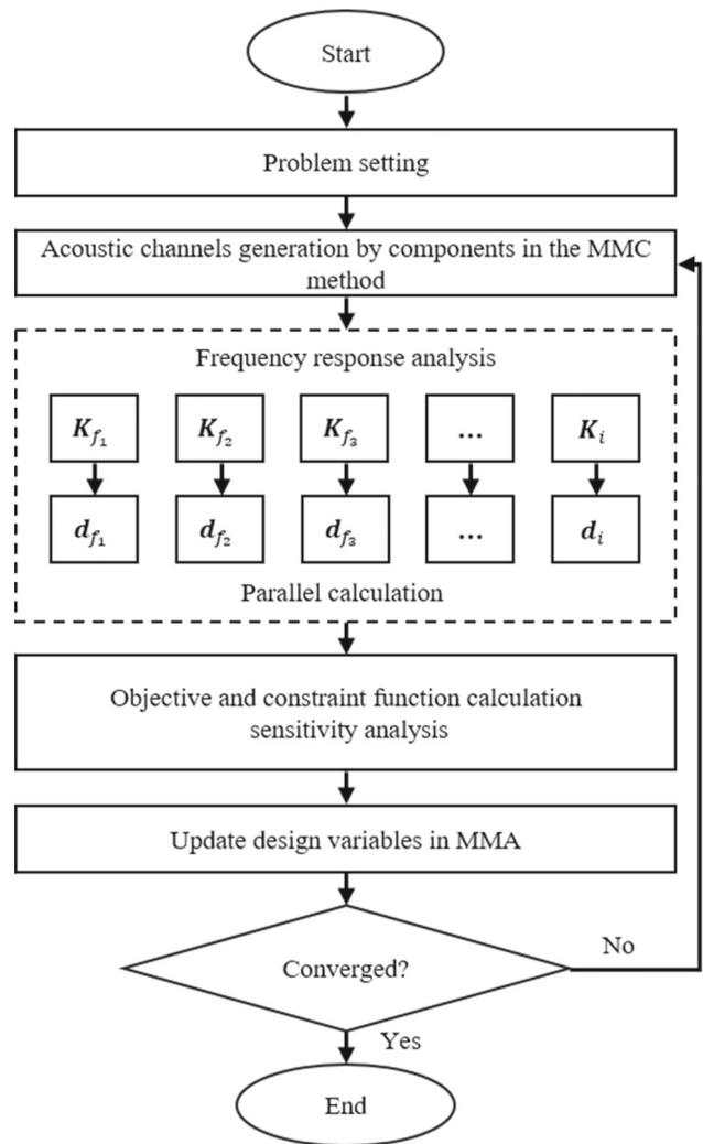
Fig. 3 Topology optimization process of acoustic–mechanical structures under the proposed MMC framework
