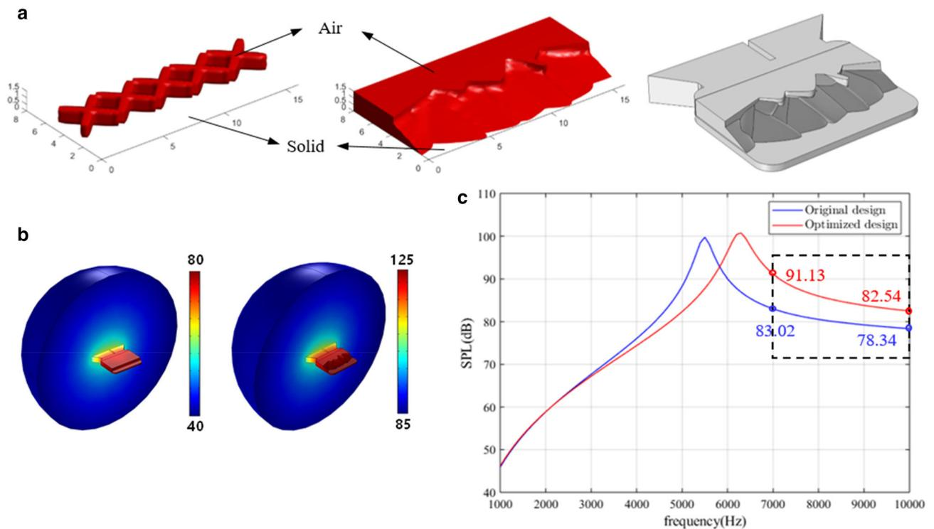
**Fig. 8** **a** The initial design of 3D acoustic channels and the optimized acoustic structure (components' plot and CAD plot), **b** distribution of SPL (dB) of the 3D cavity structure at  $f=7000$  Hz: original design
