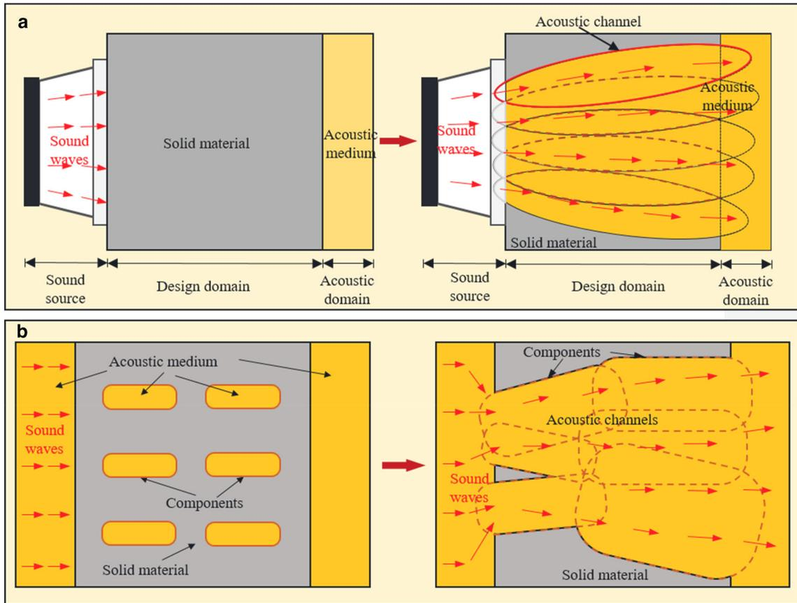
**Fig. 1** **a** The basic idea of topology optimization for acoustic–mechanical structures, **b** the basic idea of topology optimization for acoustic–mechanical structures via MMC
