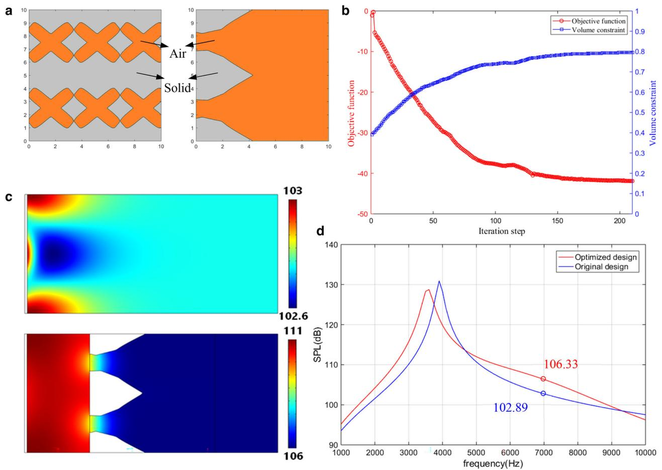
**Fig. 5** **a** The initial design and final optimized design of acoustic channels, **b** the iteration history of objective functional  $I_1$  and volume constraint, **c** distribution of SPL (dB) of the 2D cavity structure at
