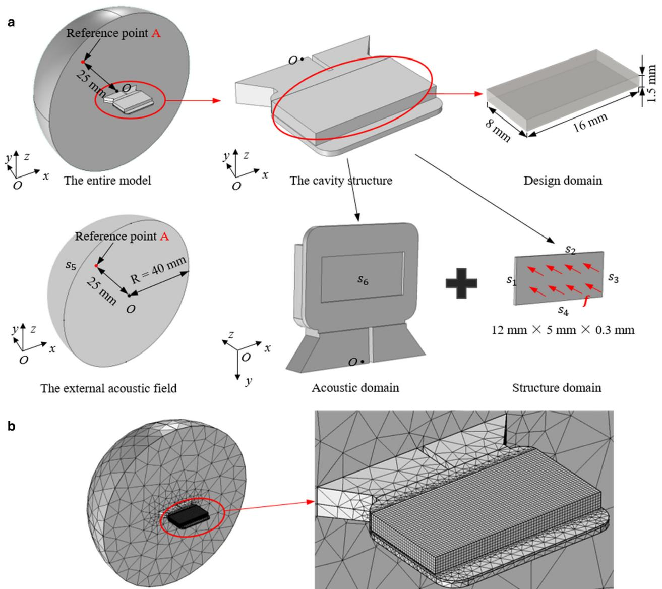
**Fig. 7** **a** A 3D cavity structure, **b** finite element mesh of the entire model
