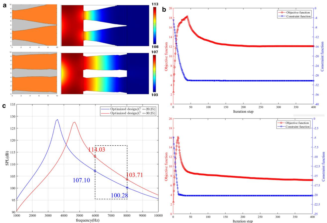
**Fig. 6** **a** The final optimized designs and the corresponding distributions of SPL (dB) of the 2D cavity structure:  $\bar{C} = -30.25$  (up) and  $\bar{C} = -20.25$  (down), **b** the iteration history of the objective function and the
