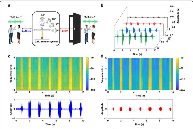
**Fig. 6 Evaluation of the performance of the sensor system. a** Schematic diagram of the speech acquisition test at different distances (10 cm and 9 m). **b** Response curve of the sensor at 0–90°. **c**, **d** Time-domain and spectrogram diagrams of the signal reconstructed by the CaF<sub>2</sub> system at distances of 10 cm and 9 m, respectively
