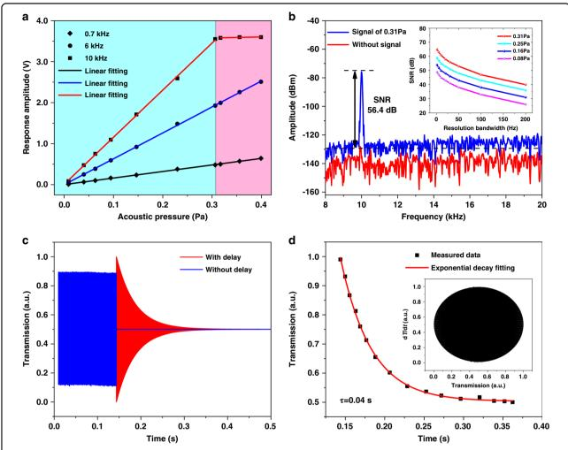
**Fig. 4 Evaluation of the performance of the sensor device. a** Variation in the response amplitude with the acoustic pressure at different frequencies with errors. **b** Frequency domain spectrum of an acoustic signal at 10 kHz and without signal. The inset shows the relationship between *SNR* and *BW* at different  $P_{\text{applied}}$ . **c** The delay response curve when the loaded signal disappears. **d** Exponential decay fitting of the delay curve
