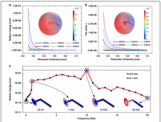
Fig. 1 Structural optimization and frequency response by simulation. a, b The variation in the radius and strain at different radii and thicknesses. The insets show the change in the radius and strain when the radius is 5.0 mm, and the thickness is 0.1 mm at 1 Pa. c The frequency response characteristics of the 7-shaped CaF<sub>2</sub> resonator system
