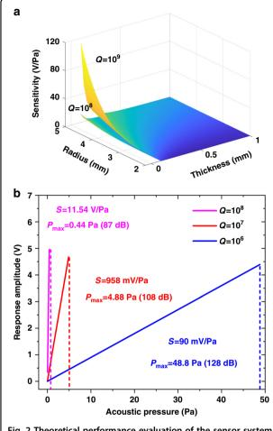
**Fig. 2 Theoretical performance evaluation of the sensor system. a** The theoretical sensitivity at different radii and thicknesses. **b** The relationship between the sensitivity and the maximum detectable acoustic pressure ( $P_{\text{max}}$ ) at different Q
