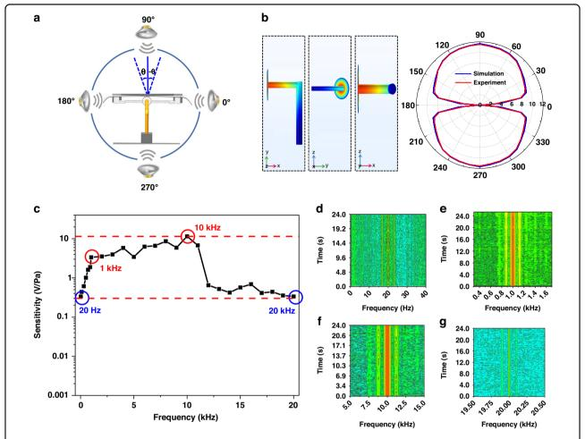
Fig. 5 Characterization of the vectorial and frequency response of the sensor. a Schematic diagram of vector testing. **b** Directivity diagram of the 7-shaped CaF<sub>2</sub> resonator structure at 10 kHz obtained by a simulation and experiment. **c** The frequency response curve of the proposed sensor. **d**–**g** Frequency response of the acoustic sensor at 20 Hz, 1 kHz, 10 kHz, and 20 kHz frequencies
