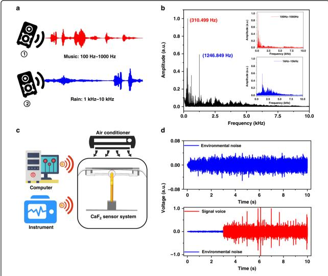
**Fig. 7 Application of the CaF<sub>2</sub> resonator sensing system in speech recognition and separation. a** Experimental setup for the simultaneous playing of different music segments. **b** The frequency-domain diagram of the signal reconstructed by the CaF<sub>2</sub> system. **c** Schematic diagrams of various background noises. **d** The voltage comparison between environmental noise and signal voice
