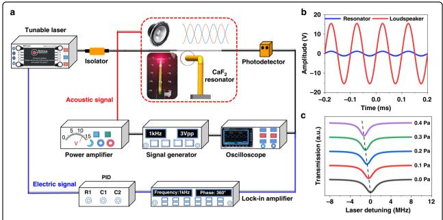
Fig. 3 Performance characterization of the  $CaF_2$  resonator acoustic sensor. a Schematic measurement setup of the  $CaF_2$  resonator acoustic sensor system. b The voltage signal received by the loudspeaker and the resonator. c The shift of the resonance spectrum changes with the acoustic pressure  $(0.0-0.4 \, \text{Pa})$
