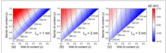
**Figure 1.**  $\Delta E$  value under different well and barrier compositions (x-y) at a well width of (a)  $L_w = 1$  nm, (b)  $L_w = 2$  nm, and (c)  $L_w = 3$  nm.
