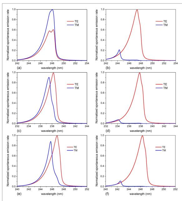
**Figure 6.** Normalized spontaneous emission rate spectra of the  $Al_yGa_{1-y}N/Al_xGa_{1-y}N/Al_yGa_{1-y}N$  quantum structures. The carrier concentrations in the QW are set to be  $1\times10^{18}$  cm $^{-3}$ . (a)  $x=0.6,y=0.888,L_w=2$  nm, unstrained; (b)  $x=0.6,y=0.888,L_w=2$  nm, strain of -0.5%; (c)  $x=0.6,y=0.888,L_w=1$  nm, unstraind; (d)  $x=0.6,y=0.888,L_w=1$  nm, strain of -0.5%; (e)  $x=0.6,y=0.888,L_w=1$  nm, unstrained; (f)  $x=0.6,y=0.888,L_w=2$  nm, strain of -0.5%.
