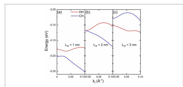
**Figure 2.** Valence subband structures of Al $_{0.888}$ Ga $_{0.112}$ N/Al $_{0.6}$ Ga $_{0.4}$ N/Al $_{0.888}$ Ga $_{0.112}$ N single well quantum structure with a different quantum well widths of (a)  $L_w = 1$  nm, (b)  $L_w = 2$  nm, and (c)  $L_w = 3$  nm, respectively.
