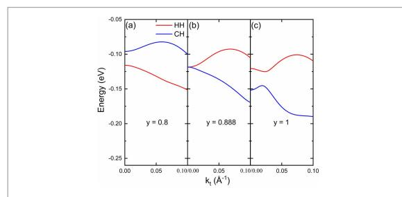
$\textbf{Figure 3.} \ \ Valence \ subband \ structures \ of \ Al_yGa_{1-y}N/Al_{0.6}Ga_{0.4}N/Al_yGa_{1-y}N \ single \ well \ quantum \ structure \ with \ well \ width \ of \ 2 \ nm \ at \ different \ barrier \ Al \ contents \ of \ (a) \ y=0.8, (b) \ y=0.888, \ and \ (c) \ y=1, \ respectively.$
