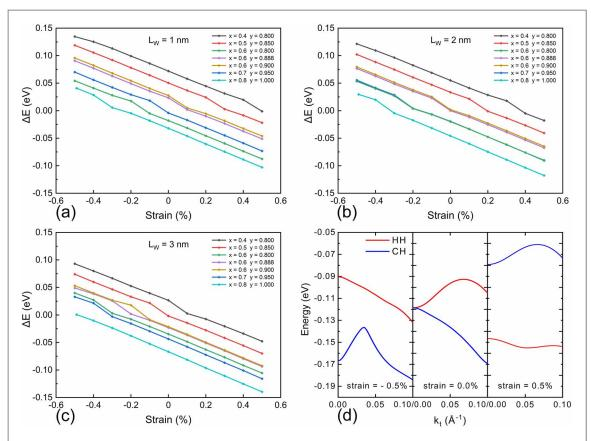
**Figure 4.** The  $\Delta E$  variation trends with strain of some different  $Al_yGa_{1-y}N/Al_xGa_{1-x}N/Al_yGa_{1-y}N$  quantum structures at the well width of (a)  $L_w=1$  nm, (b)  $L_w=2$  nm, and (c)  $L_w=3$  nm, respectively. (d) Valence subband structures of the  $Al_{0.888}Ga_{0.112}N/Al_{0.6}Ga_{0.4}N/Al_{0.888}Ga_{0.112}N$  quantum structure with  $L_w=2$  nm under different strains.
