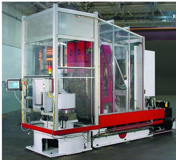
Flexible Adaptive Servohydraulic Technology (FAST) machining center Eric developed in his father's company
