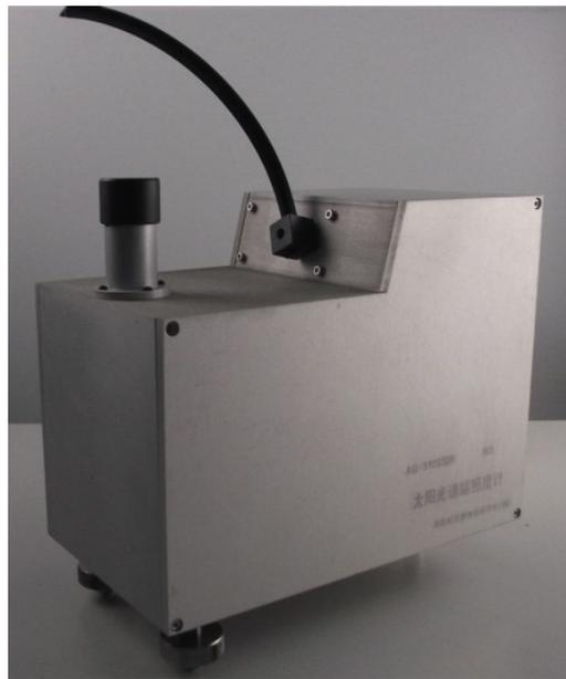
**Figure 6.** AG-512 SSIR Solar Spectroradiometer.
