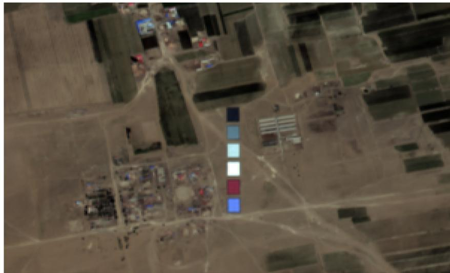
**Figure 4.** The spatial layout of the radiometric calibration tarps in this study at Baotou site.
