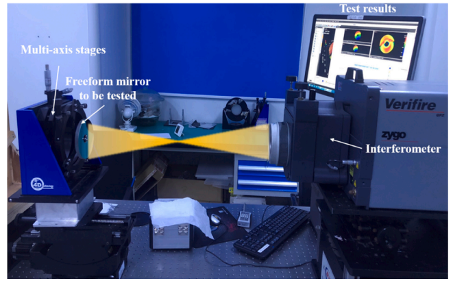
Fig. 10. Interferometer measures the freeform surface of the mirror.
