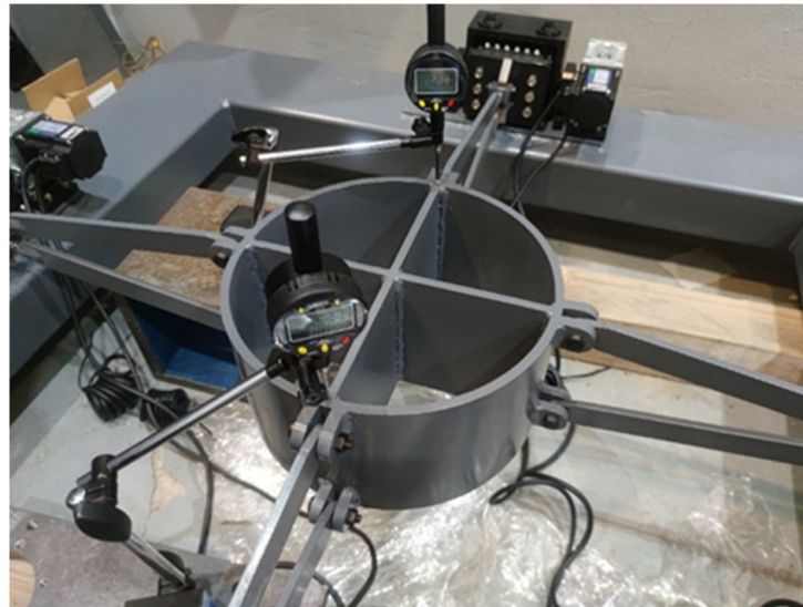
Figure 12. Deflection accuracy test with micrometers.
