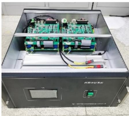
Figure 13. The servo controller and driver of 2.5-m-wide field survey telescope.
