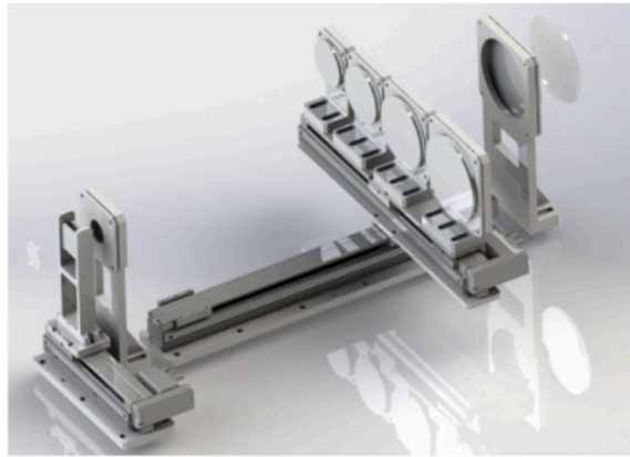
Fig. 4. Schematic of the laser shock beam shaping system.
