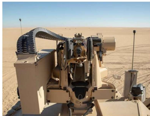
Figure 1. MLIDS integrated defense system.
