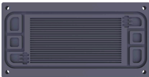
Fig. 1. (a) Schematic showing the single cell test bench. (b) Single cell PCB assembly used for current density and temperature distribution measurements. (c) Anode flow field. (d) Cathode flow field.
