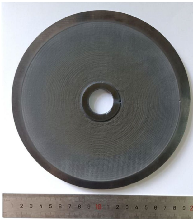
Fig. 14 Aspherical RB-SiC surface processed by abrasive water jet milling
