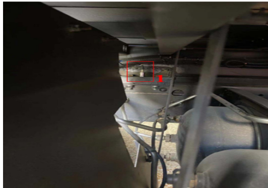
Fig. 23. Schematic diagram of test points for system vibration isolation efficiency test.
