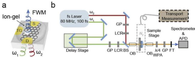
**Fig. 1.** Experimental setup. (a) Illustration of helicity-selective FWM in an ion-gel-gated graphene device. D: drain electrode, S: source electrode, TG: top gate electrode. (b) Illustration of the experimental setup for two-color four-wave mixing measurement. GP: Glan–Thompson polarizer, LCR: liquid-crystal retarder, BS: beam splitter, OB: objective, FT: filter, APD: avalanche photodiode.  $\Omega_1$ : 1.192 eV,  $\Omega_2$ : 0.954 eV.
