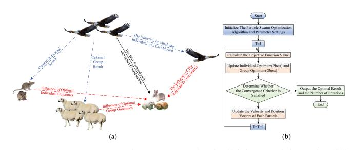
**Figure 6.** Particle swarm optimization algorithm: (**a**) the basic principle diagram of PSO; (**b**) basic flow chart of PSO.
