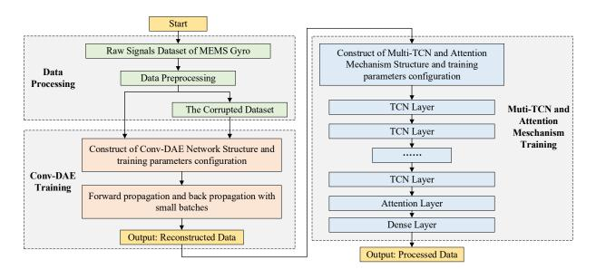
Figure 5. Multi-layer deep learning network combination model structure diagram.
