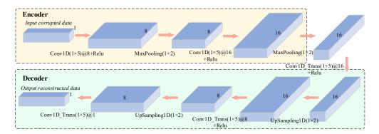
Figure 2. The detailed structure of the denoising autoencoder used in the experiment.
