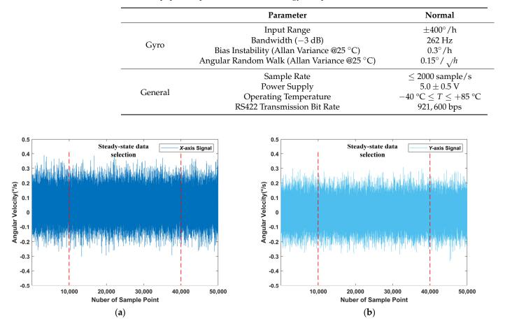
Figure 9. Raw gyroscope data under static conditions. (a) X-axis raw signal; (b) Y-axis raw signal.
