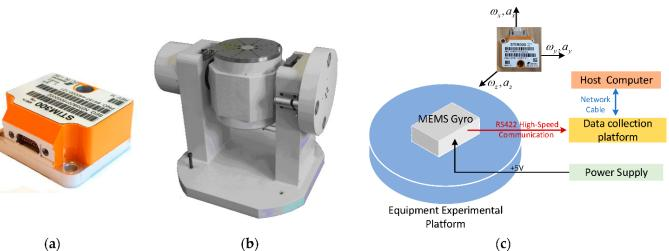
Figure 8. Equipment testing device. (a) STIM300 IMU; (b) static IMU data collection system; (c) data acquisition procedure.
