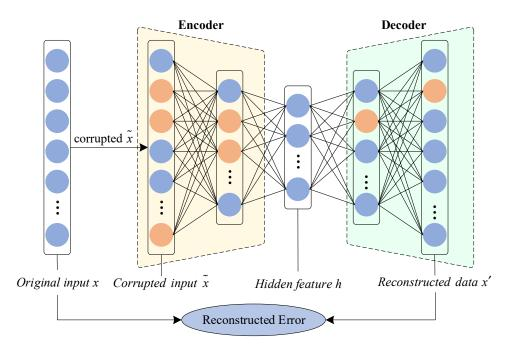
Figure 1. The overall structure of a denoising autoencoder.
