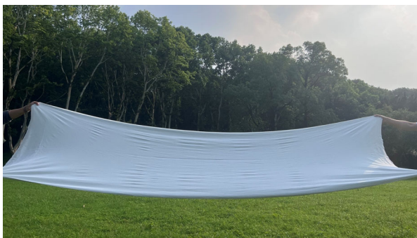
Massive-fabricated passive cooling metafabric based on modified polyester fibers (the latest result)
