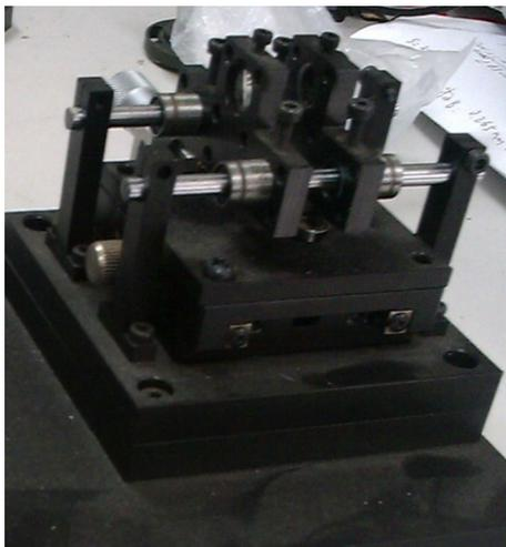
Fig. 10 Zoom collimating lens
