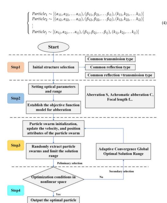
Figure 1. Multi-level screening model based on adaptive particle swarm optimization.
