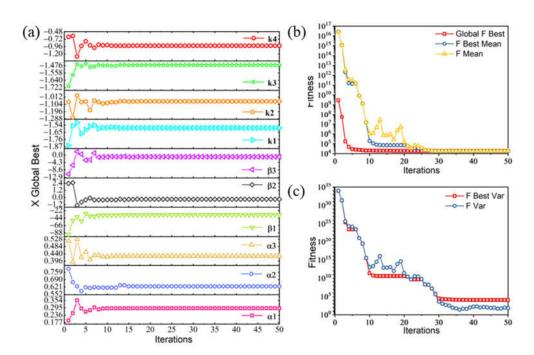
**Figure 5.** Search results of APSO algorithm for four-reflection system; (a) the parameter search results of the objective function; (b) the optimization results of objective function value of APSO algorithm; (c) the optimization results of objective function variance value of APSO algorithm.
