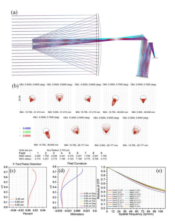
Figure 9. The rear-reflection path 2. (a) Optical layout diagram. (b) Spot diagram. (c) Distortion of the different wavelengths. (d) Field curvature of the different wavelengths. (e) Modulation transfer function diagram.
