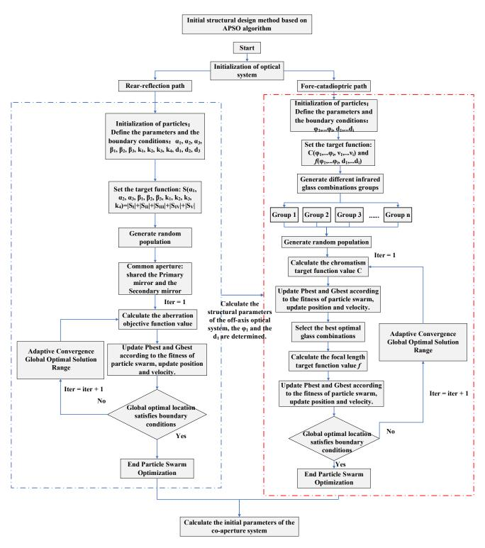
Figure 3. Flow chart of APSO algorithm.
