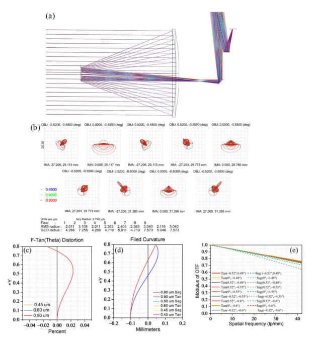
**Figure 8.** The rear-reflection path 1. (a) Optical layout diagram. (b) Spot diagram. (c) Distortion of the different wavelengths. (d) Field curvature of the different wavelengths. (e) Modulation transfer function diagram.
