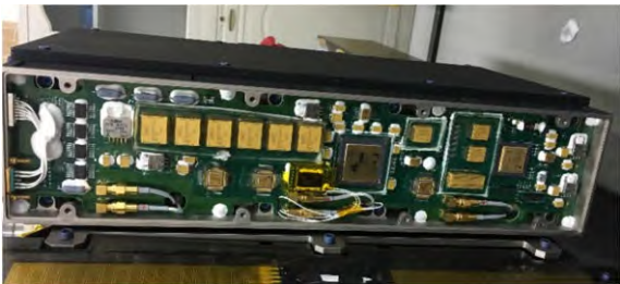
图 6 高分相机图像存储电子学系统 Fig. 6 Image storage and processing electronics system of high resolution camera
