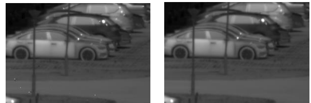
(a) 关闭盲元补偿功能 (b) 开启盲元补偿功能 (a) Turn off the blind pixel compensation function (b) Turn on the blind pixel compensation function
