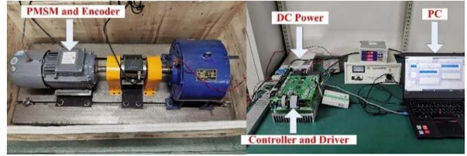
Fig. 19. Photograph of the experimental platform.
