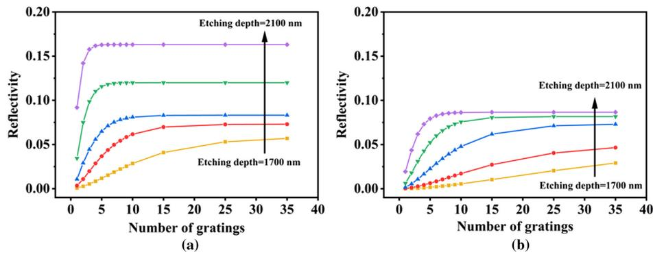
**Fig. 4.** Variation of Bragg grating reflection spectrum with the number of gratings  $N$  under different etching depths of (a) the symmetrical epitaxial structure and (b) the asymmetrical epitaxial structure.
