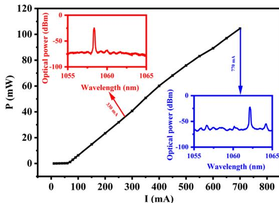
**Fig. 6.** Relationship between the injected current and output power. Upper left illustration shows the spectrum at 330 mA, and the lower right illustration shows the spectrum at 770 mA.
