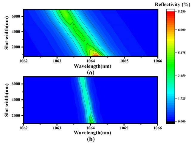
**Fig. 2.** Variation of Bragg grating reflection spectrum with slot width of (a) the symmetrical epitaxial structure and (b) the asymmetrical epitaxial structure.  $N$  is set to 200.
