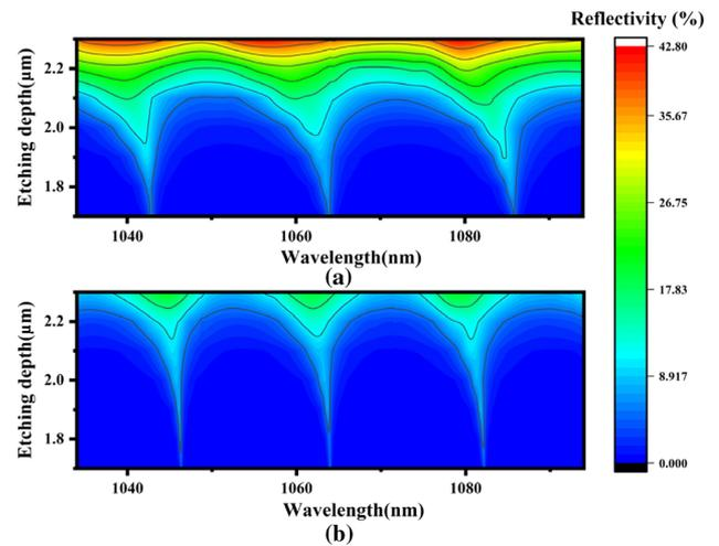
**Fig. 3.** Variation of Bragg grating reflection spectrum with slot depth of (a) the symmetrical epitaxial structure and (b) the asymmetrical epitaxial structure.  $N$  is set to 200.
