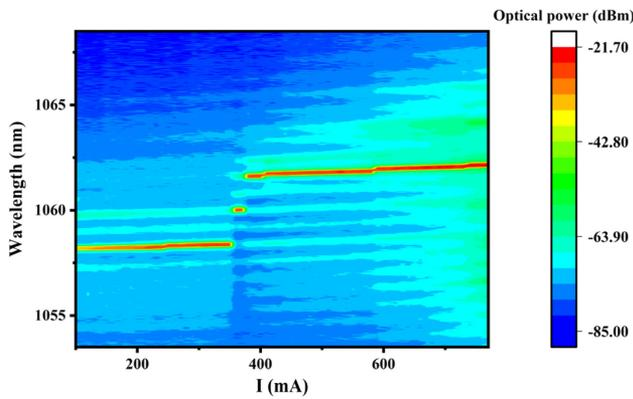
**Fig. 5.** Spectrogram of different injection currents.
