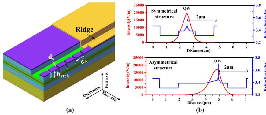
**Fig. 1.** (a) 3D cross-section drawn along the optical oscillation direction of the DBR laser. (b) Electric field intensity and refractive index distribution along the epitaxial direction of the symmetrical and asymmetrical structure.
