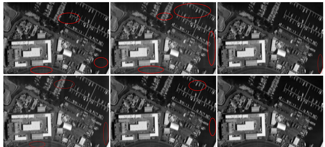
Figure 13. Destriping result of the real remote sensing image (From left to right , the first row are the destriping results of SLD, LRSID and TVGS; the second row are the destriping results of GSLV, HTVLR and the Proposed).
