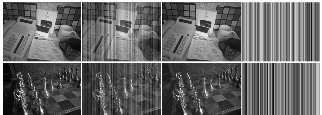
Figure 9. Destriping results of non-remote sensing images (From top to bottom are the different images. From left to right are the original image, degraded image, the restored image and stripes separated by the proposed model).
