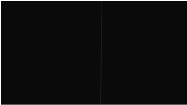
Fig. 12 Experimental results obtained with CMOS by loading Figs. 10 and 11 into slm1 and SLM2 in the 4f system, respectively, a bright line in the vertical direction is obtained because only the horizontal filtering is done
