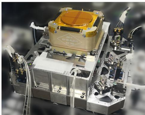
Fig. 3. Optical photograph of the Taiji-1 OB (assembled with the GRS).
