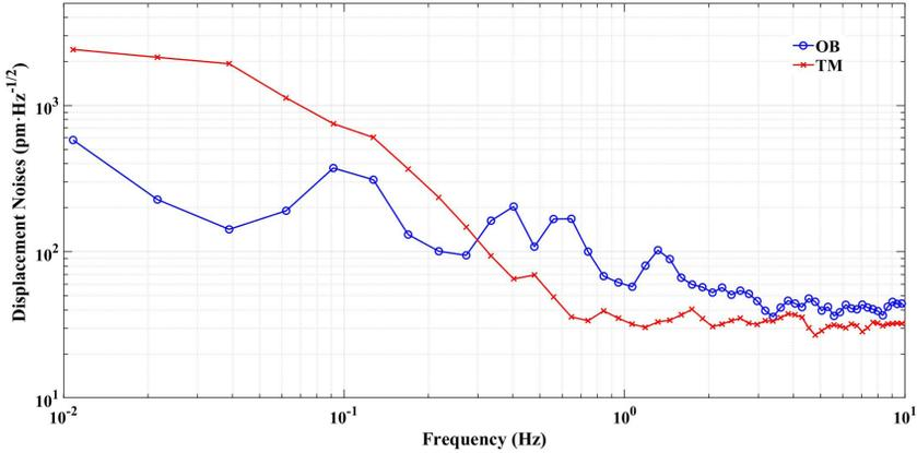
Fig. 5. Typical results of Taiji-1 in orbit (backup part).
