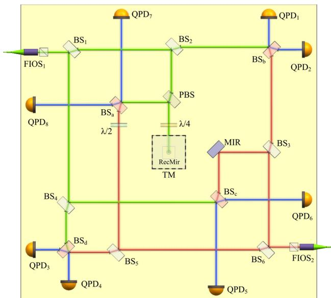
Fig. 1. The optical layout of the OB of the Taiji-1 experimental satellite. FIOS: fiber injector optical subassembly; BS: beam splitter; QPD: quadrant photo detector; PBS: polarization beam splitter; TM: test mass; MIR: mirror and RecMir: rectangle mirror.
