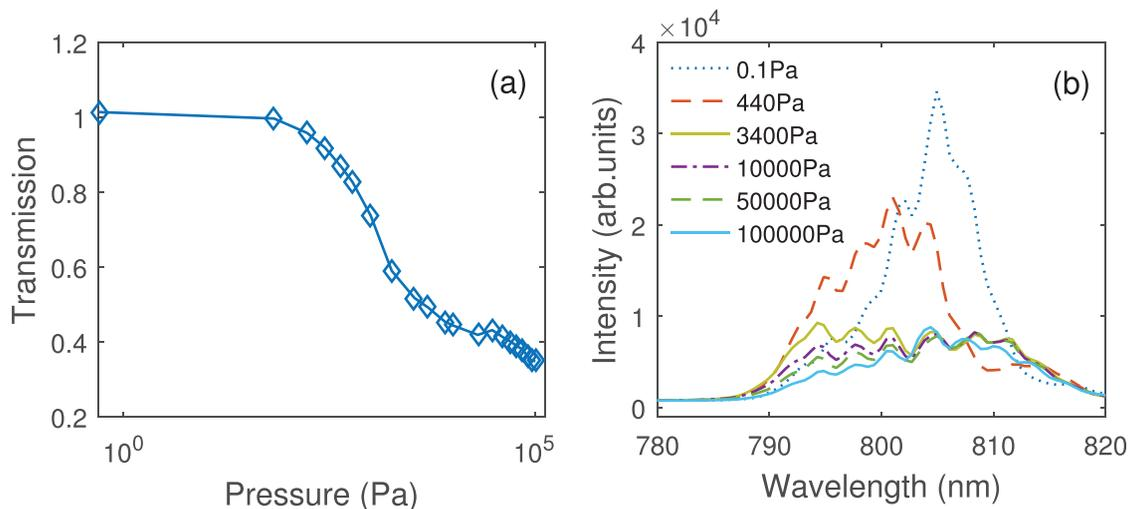
**FIG. 5.** (a) Variation of the transmission (blue diamond line) for 800 nm with pressure when the incident laser energy is 2.5 mJ. (b) Spectra measured at different pressures after the transmitted laser energy is detected.
