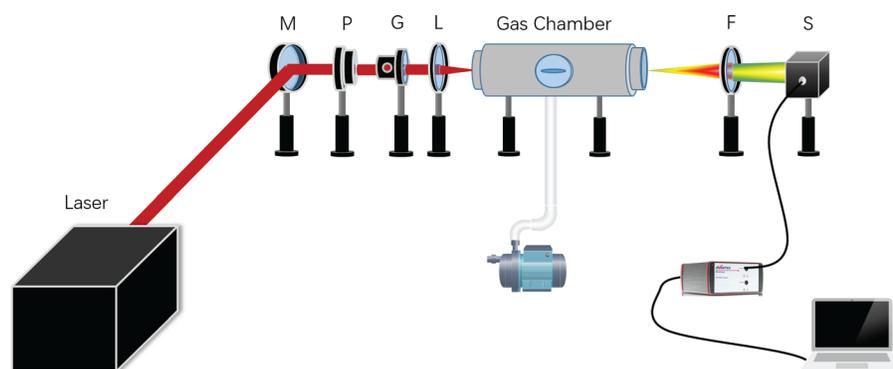
FIG. 1. Schematic of experimental setup: Laser: femtosecond laser, M: planar mirror, P: half wave plate, G: Glan prism, L: focusing lens ( $f=400$  mm), F: 800 nm filter, and S: integrating sphere.
