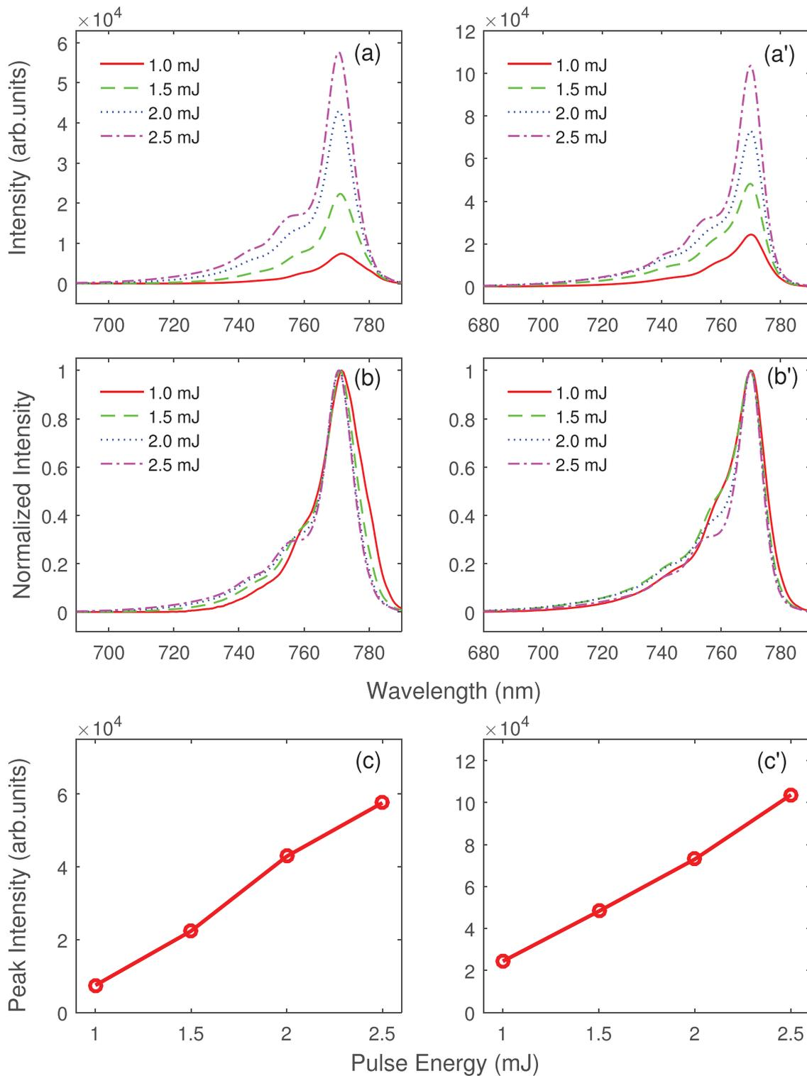
**FIG. 4.** (a) Spectra measured at 40 000 Pa and (b) normalized spectra measured at 40 000 Pa under different pulse energies, and (c) variation of the peak spectral intensity with pulse energy. (a') Spectra and (b') normalized spectra under different pulse energies at a fixed pressure of 100 000 Pa, and (c') variation of the peak spectral intensity with pulse energy.
