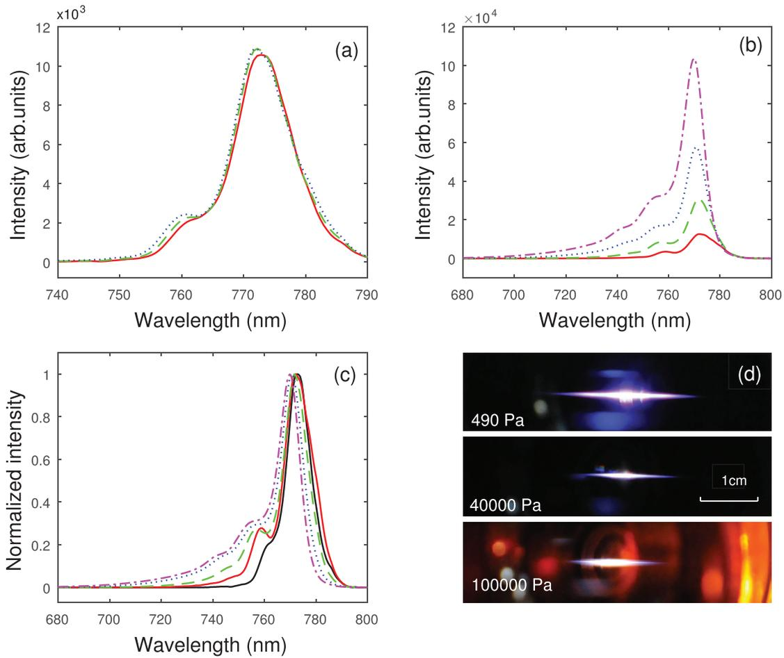
**FIG. 2.** Spectra measured at  $E_{in}= 2.0$  mJ when the pressure is (a) lower and (b) higher than 1000 Pa, (c) normalized spectra. (d) Pictures of the luminous region taken from the middle quartz window when the pressure in the gas chamber is 490, 40 000, and 100 000 Pa, respectively.
