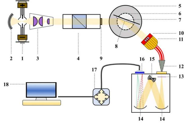
Fig. 1. Schematic of the designed ellipsometric system. 1: continuous light source. 2: spherical mirror. 3: light-collimating lens. 4: fixed polarizer. 5: rotating stage. 6: sample rotator. 7: sample holder. 8: sample. 9: incident window. 10: integrated analyzer. 11: fiber-coupler array. 12: optical-fiber adapter. 13: filter. 14: spherical mirrors. 15: plane grating. 16: 2-D CCD detector. 17: controller. 18: computer.
