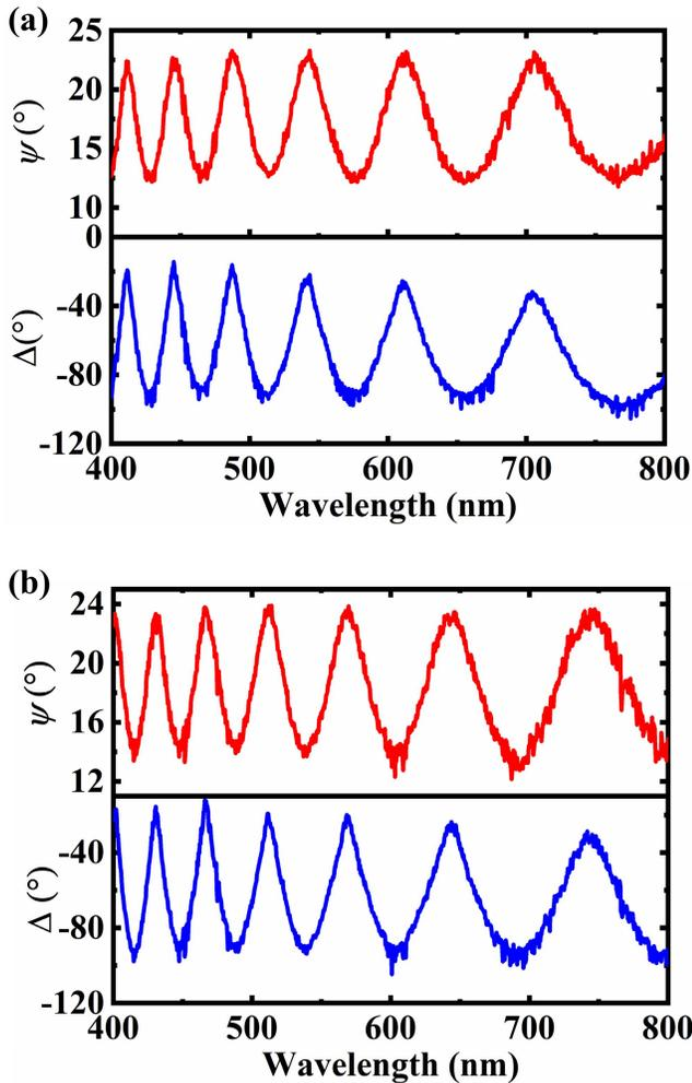
Fig. 9. Ellipsometric parameters of tantalum-pentoxide film prepared on a glass substrate, measured at an incident angle of  $70^\circ$  in the 400–800 nm wavelength range with the suggested ellipsometer. (a) Before and (b) after heating.
