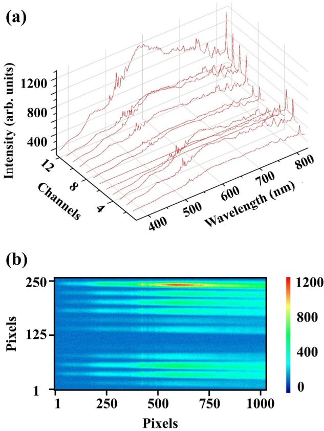
Fig. 5. (a) Spectra of 12 polarization channels for Au bulk, measured at an incident angle of  $70^\circ$ . (b) Corresponding image pattern for the spectra showing the distribution of light intensity for 12 optical channels.
