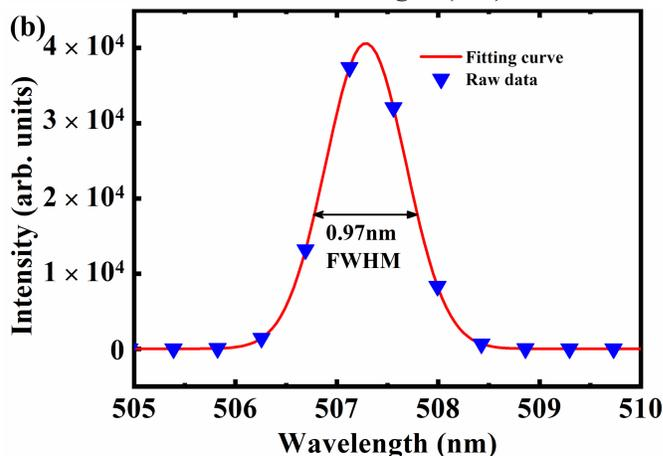
Fig. 4. (a) Spectral lines of mercury lamp measured by the spectrometer. (b) Magnified view of the well-resolved spectral line and the fitting curve at 507.3 nm.
