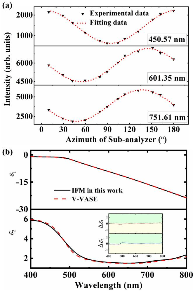
Fig. 7. (a) Comparison between 12 raw data of light intensity and fitting curves at three typical wavelengths in the spectral range. (b) Dielectric functions of the Au bulk sample measured with the developed ellipsometer in this work and the V-VASE (J. A. Woollam), with the differences shown in the inset.
