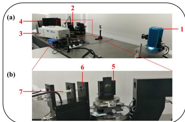
Fig. 2. (a) Photograph of the configuration of system. 1: light source. 2: ellipsometric rotating system. 3: spectrum acquisition system. 4: computer control system. (b) Enlarged photograph of the ellipsometric rotating system. 5: sample stage. 6: integrated analyzer. 7: fiber-coupler array.
