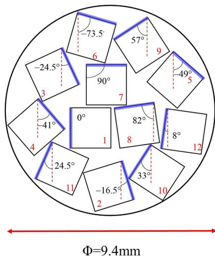
Fig. 3. Schematic of the 12 subanalyzers designed in a dimension of 9.4 mm.
