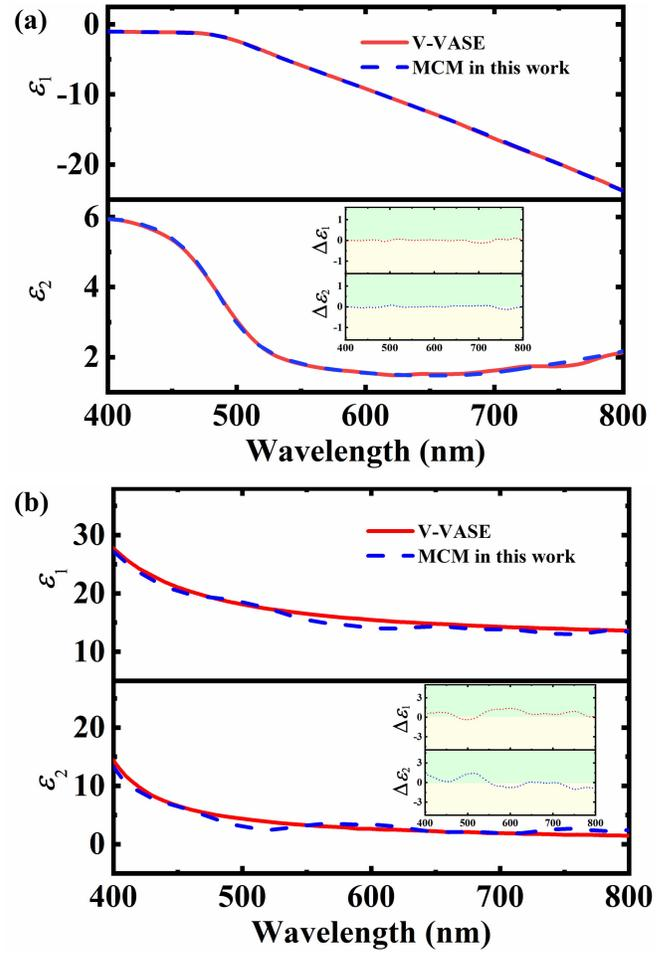
Fig. 8. Measured dielectric functions at an incident angle of 70° of the (a) Au and (b) Si bulk samples, compared with those with the V-VASE (J. A. Woollam), with the differences shown in the insets.
