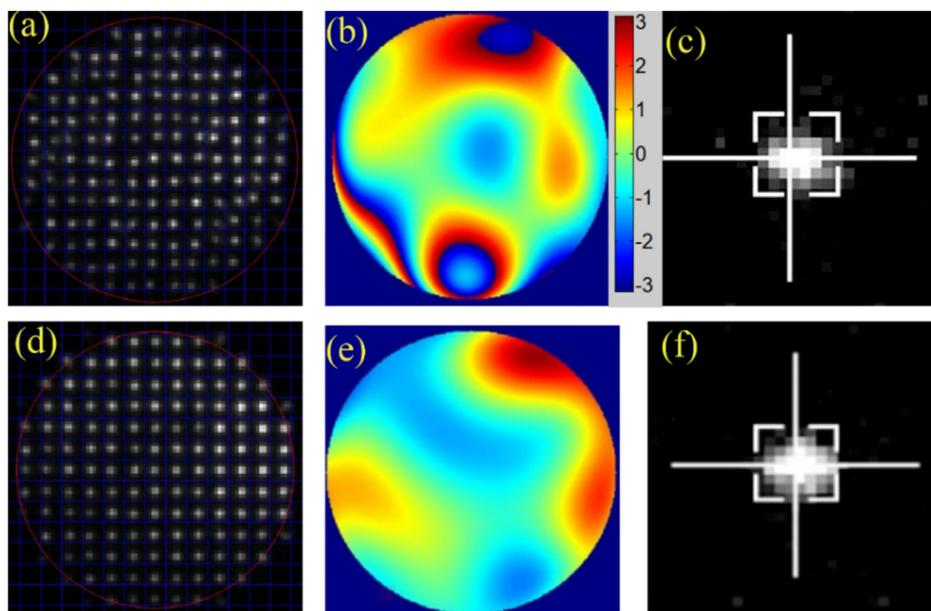
Fig. 9. Static turbulence with correction: the upper part presents the correction results for the SPGD method with the correlativity of 0.81 and the (a) Spot diagram, (b) Wavefront, and (c) Image. The lower part presents the correction results with SH WFS and the (e) Spot diagram, (f) Wavefront and (g) Image.
