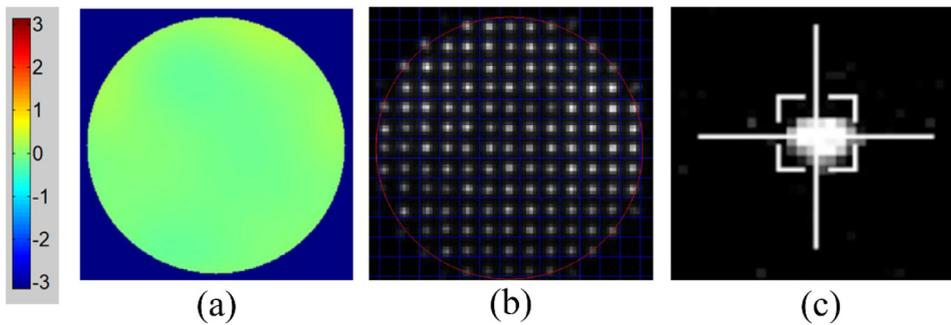
Fig. 6. AOS without the aberrations: (a) Wavefront; (b) Reference spot diagram; (c) Image.
