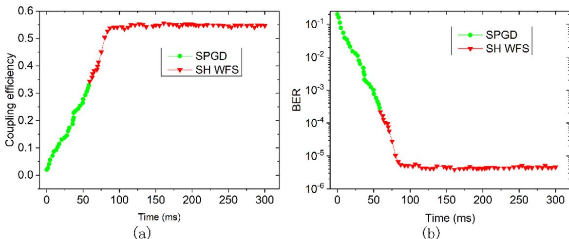
Fig. 11. Communication performance: the coupling efficiency (a) and BER (b) as functions of correction time.
