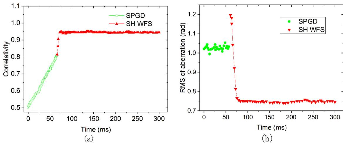
Fig. 10. Correction of dynamic turbulence: the correlativity (a) and RMS of corrected wavefront (b) as functions of the correction time.
