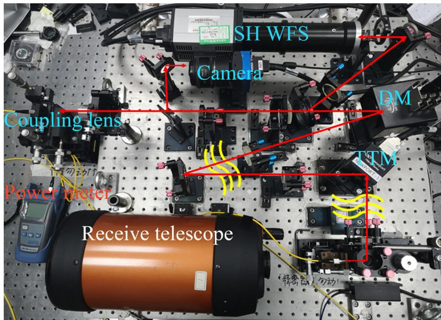
Fig. 5. Optical layout for AOS of the FSOC.
