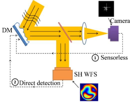
Fig. 1. Configuration for the combination of the wavefront sensorless and SH WFS modes.
