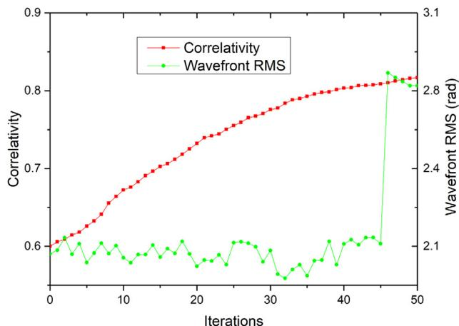
Fig. 8. Correlativity and RMS of the measured wavefront as functions of iterations.
