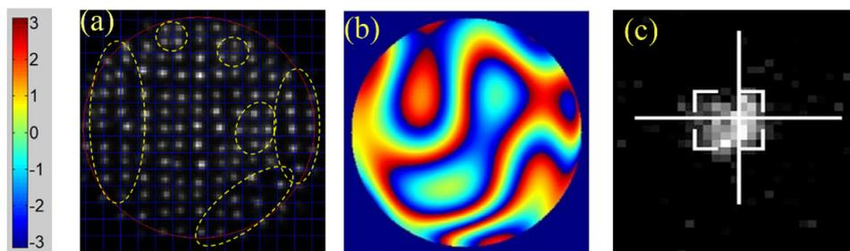
Fig. 7. AOS with static turbulence: (a) Spot diagram; (b) Measured wavefront by SH WFS; (c) Image.
