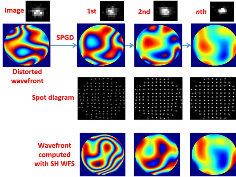
Fig. 3. Simulation of the correction process with the wavefront sensorless mode: the input image is produced with a distorted wavefront. The first row presents the images calculated with the retrieved wavefronts at the second row, and the third row presents the spot diagrams computed according to the retrieved wavefronts. The detected wavefront by SH WFS is calculated with the corresponding spot diagram.
