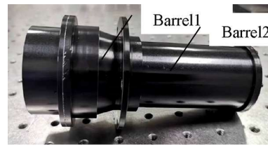
Figure 6 Optimized structure of the lens
