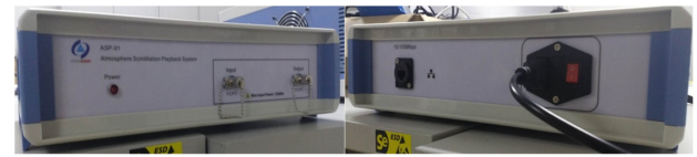
Fig. 12. Photo of the atmosphere scintillation playback system.
