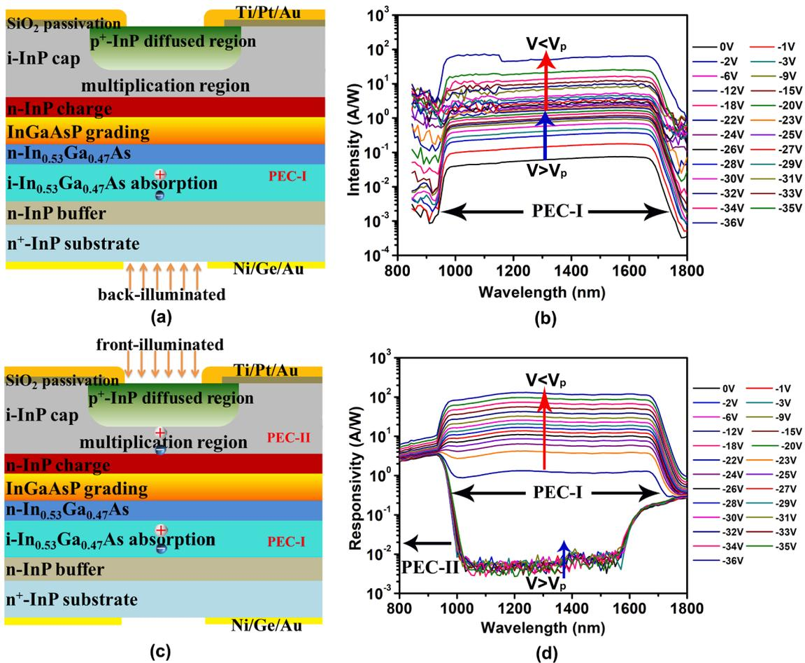
Fig. 3. The comparison of working process and spectral characteristic between the front illumination and the back illumination for the InGaAs/InP APD. (a) The spectral characteristics under front illumination and (b) its related illustration of working process. (c) The spectral characteristics under back illumination and (d) its related illustration of working process.
