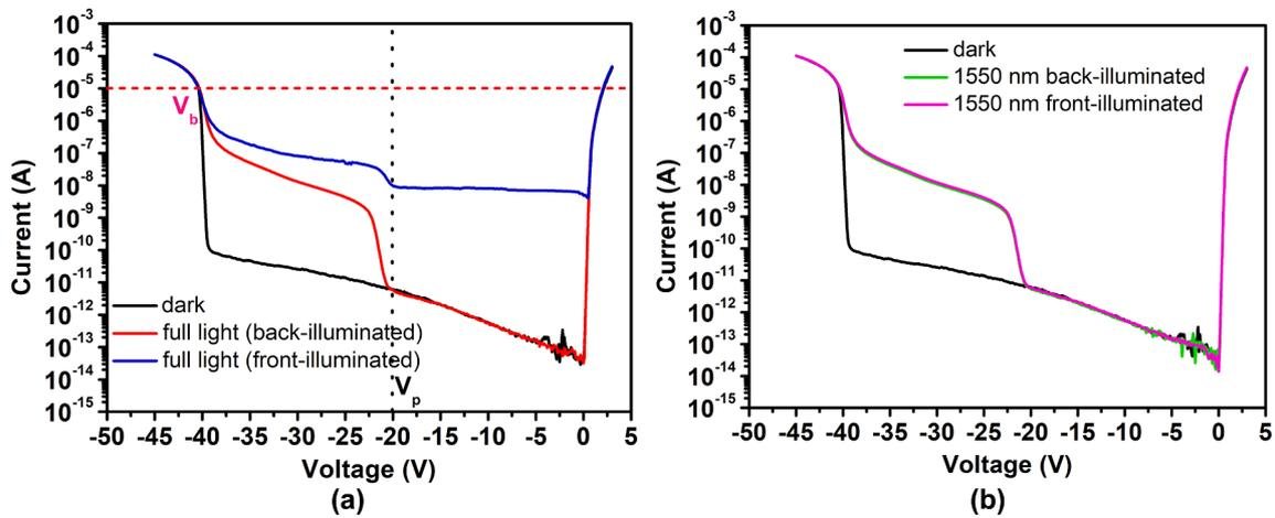
Fig. 2. (a) Comparison of electrical properties under dark, back-illuminated, and front-illuminated conditions using a full-spectrum light source. (b) Comparison of electrical properties under dark, back-illuminated, and front-illuminated conditions using a 1550-nm-wavelength light.
