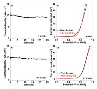
**Fig. 4** (a) Chronoamperometric measurement in 1 KOH. (b) OER polarization curves without iR-compensation. (c) Chronoamperometric measurement in 0.1 KOH. (d) OER polarization curves.
