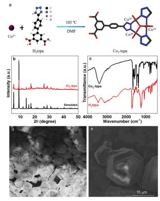
Fig. 1 (a) Synthetic procedure of  $Co_2$ -tzpa. (b) XRD patterns of experimental and simulated  $Co_2$ -tzpa. (c) FT-IR spectra of H<sub>3</sub>tzpa and Co<sub>2</sub>-tzpa. (d and e) SEM images of  $Co_2$ -tzpa with different amplifications.
