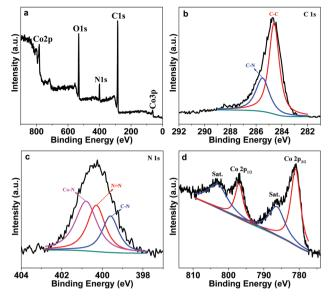
Fig. 2 (a) XPS survey spectrum. (b–d) High resolution XPS spectra for (b) C 1s, (c) N 1s, and (d) Co 2p regions of  $Co_2$ -tzpa.
