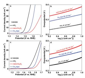
**Fig. 3** (a) OER polarization curves and (b) Tafel plots in 1 M KOH. (c) OER polarization curves and (d) Tafel plots in 0.1 M KOH.
