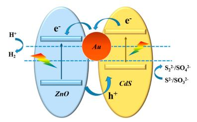
**Figure 9.** Schematic illustration of charge transfer process and gas evolution mechanism of ZnO/Au/CdS sample.
