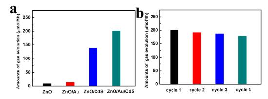
**Figure 8.** (a) The amounts of gas evolution of the ZnO, ZnO/Au, ZnO/CdS and ZnO/Au/CdS samples (100 mg of catalyst for 4 h); (b) the cycling stability of the ZnO/Au/CdS photocatalyst (4 h as a cycle).
