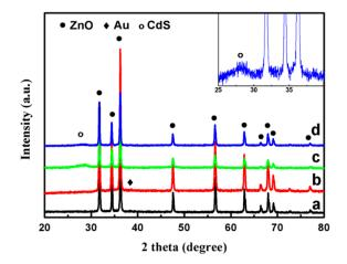
**Figure 1.** XRD patterns of (**a**) ZnO; (**b**) ZnO/Au; (**c**) ZnO/CdS; and (**d**) ZnO/Au/CdS samples. Inset: magnification images of a portion of the XRD pattern.
