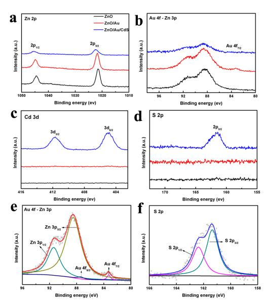
**Figure 4.** (a) Zn 2p, (b) Au 4f-Zn 3p, (c) Cd 3d, and (d) S 2p peaks in XPS spectra of ZnO, ZnO/Au and ZnO/Au/CdS samples, respectively; (e) Au 4f-Zn 3p peaks of ZnO/Au sample and (f) S 2p peaks of ZnO/Au/CdS sample.
