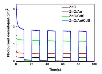
Figure 6. Transient photocurrent response of ZnO, ZnO/Au, ZnO/CdS and ZnO/Au/CdS sample.
