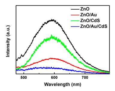
Figure 7. Photoluminescence (PL) spectra of ZnO, ZnO/Au, ZnO/CdS and ZnO/Au/CdS samples.
