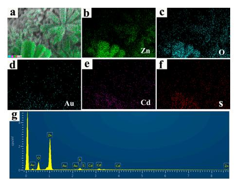
**Figure 3.** (**a**–**f**) EDS mapping images of the ZnO/Au/CdS sample; and (**g**) EDS image of the ZnO/Au/CdS sample.
