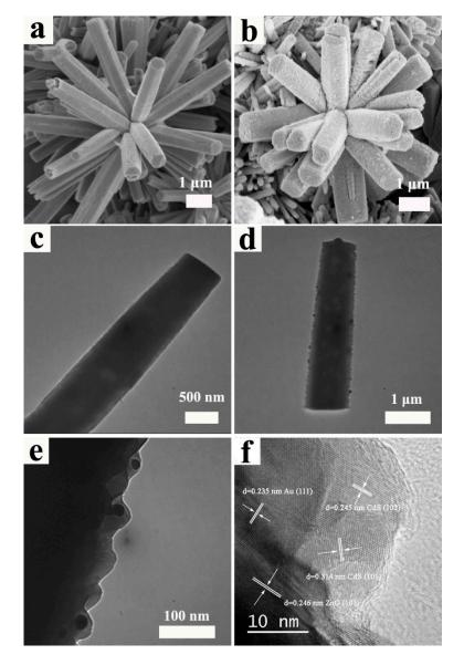
**Figure 2.** FESEM images of (**a**) ZnO sample and (**b**) ZnO/Au/CdS sample; TEM images of (**c**) ZnO sample and (**d**,**e**) ZnO/Au/CdS sample; (**f**) HRTEM image of ZnO/Au/CdS sample.
