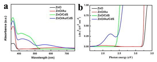
**Figure 5.** (a) UV-vis absorption spectra and (b)  $(ahv)^2$ -photon energy curves of the ZnO, ZnO/Au, ZnO/CdS, and ZnO/Au/CdS samples.
