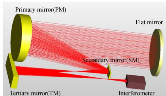
Fig. 1 Illustration of self-collimation interference optical path
