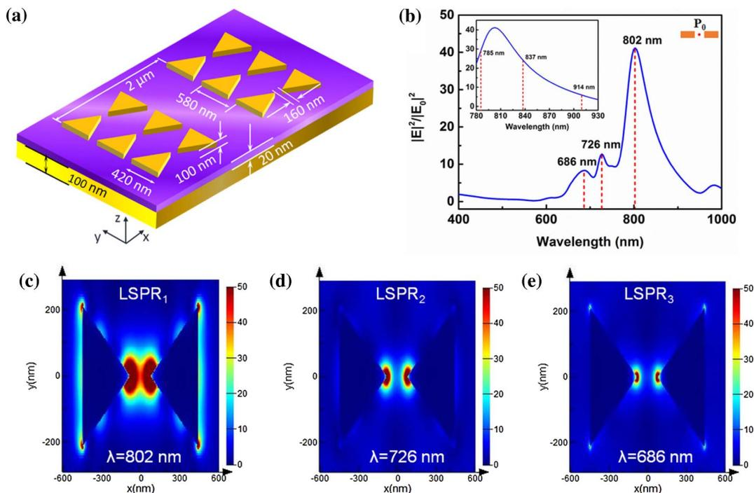
**Fig. 3.** Schematics and calculated E-field distribution of Au BNA arrays. (a) Geometrical parameters of BNA arrays with MIM structure. (b) E-field enhancement of the BNA arrays at  $P_0$  point. Inset shows the enlarged E-field enhancement spectrum range from 780 to 930 nm. (c)–(e) E-field distribution ( $|E|^2/|E_0|^2$ ) in  $x$ - $y$  plane at three LSPR modes.
