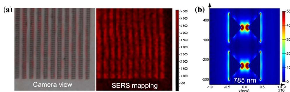
**Fig. 12.** Mapping of SERS spectrum and E-field distribution. (a) Camera view of scanning area (left side) and mapping of SERS spectrum at 1138 cm<sup>-1</sup> corresponding to the scanning area (right side). (b) Spatial E-field distribution ( $|E|^2/|E_0|^2$ ) of BNA arrays under 785 nm excitation.
