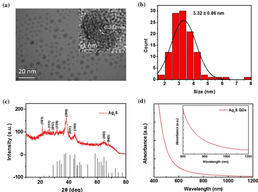
**Fig. 1.** Characterization of Ag<sub>2</sub>S QDs. (a) TEM image of Ag<sub>2</sub>S QDs (scale bar 20 nm). Inset shows an HRTEM image of a QD with a lattice spacing of 0.241 nm (scale bar 1 nm). (b) Histogram for the size distribution of Ag<sub>2</sub>S QDs with average size of 3.32 nm. (c) XRD spectrum of the Ag<sub>2</sub>S QDs with JCPDS data. (d) UV-vis-NIR absorption spectra of the Ag<sub>2</sub>S QDs.
