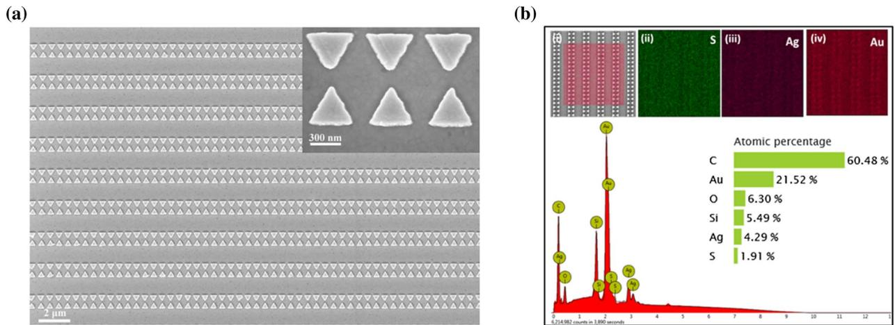
**Fig. 2.** Characterization of Au BNA arrays. (a) SEM images of the BNA arrays (scale bar 2  $\mu\text{m}$ ). Inset shows an enlarged view of three pairs of BNA (scale bar 300 nm). (b) EDS analysis of  $\text{Ag}_2\text{S}$  QDs on BNA arrays. On the top, from left to right: (i) scanned region for EDS, and elemental mapping of (ii) S, (iii) Ag, and (iv) Au. Inset shows the elemental composition of different elements in BNA arrays/ $\text{Ag}_2\text{S}$ -QDs substrate.
