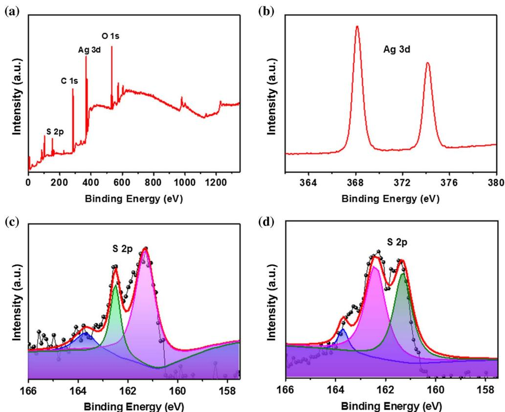
**Fig. 9.** XPS characterization of Ag<sub>2</sub>S QDs. (a), (b) Overall and Ag 3d of Ag<sub>2</sub>S coated BNA arrays, respectively. (c), (d) S 2p of Ag<sub>2</sub>S coated BNA arrays with and without PATP molecule, respectively.
