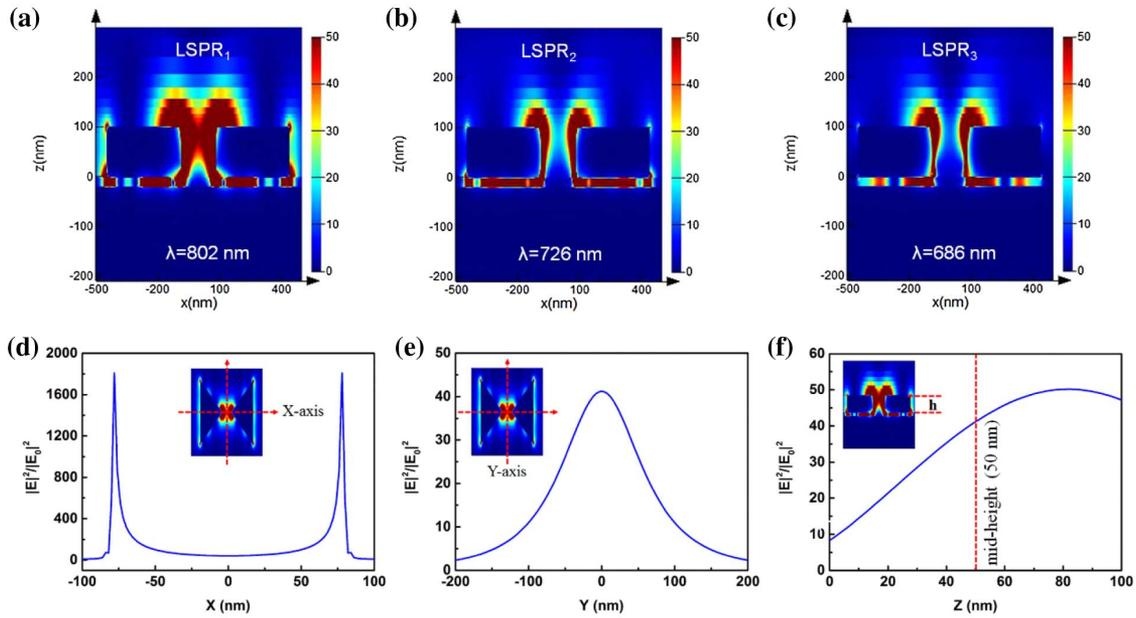
**Fig. 10.** Calculated distribution of E-field under three modes. (a)–(c) Spatial E-field distribution at a wavelength of 802 nm (LSPR<sub>1</sub>), 726 nm (LSPR<sub>2</sub>), and 686 nm (LSPR<sub>3</sub>) in the  $x$ – $z$  plane, respectively. (d)–(f) The line distribution of E-field enhancement at 802 nm (LSPR<sub>1</sub> mode) along  $x$ ,  $y$ , and  $z$  direction, respectively. Inset figures show the assumed direction of  $x$ ,  $y$ , and range of height ( $h$ ).
