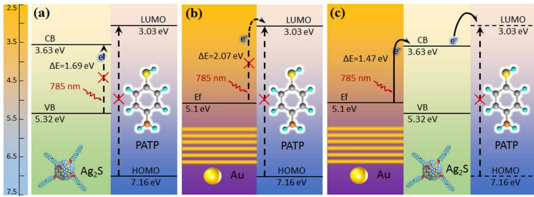
**Fig. 6.** Energy level diagram of (a) Ag<sub>2</sub>S-QDs/PATP, (b) Au-BNA/PATP, and (c) BNA/Ag<sub>2</sub>S-QDs/PATP systems under 785 nm laser excitation, respectively.
