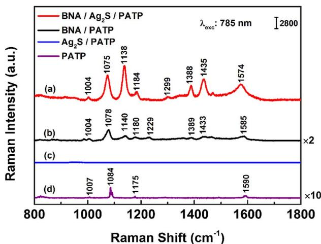
**Fig. 4.** Raman spectra of PATP molecules adsorbed on a different substrate. (a)–(c) Raman spectra of PATP molecules adsorbed on Ag<sub>2</sub>S QDs coated BNA arrays (red curve), BNA arrays (black curve), and Ag<sub>2</sub>S QDs (blue curve), respectively. (d) Raman spectrum of PATP powder as reference. The spectra were collected under 785 nm laser excitation. Raman spectra are shifted compared to each other along the  $y$  axis for better viewing.
