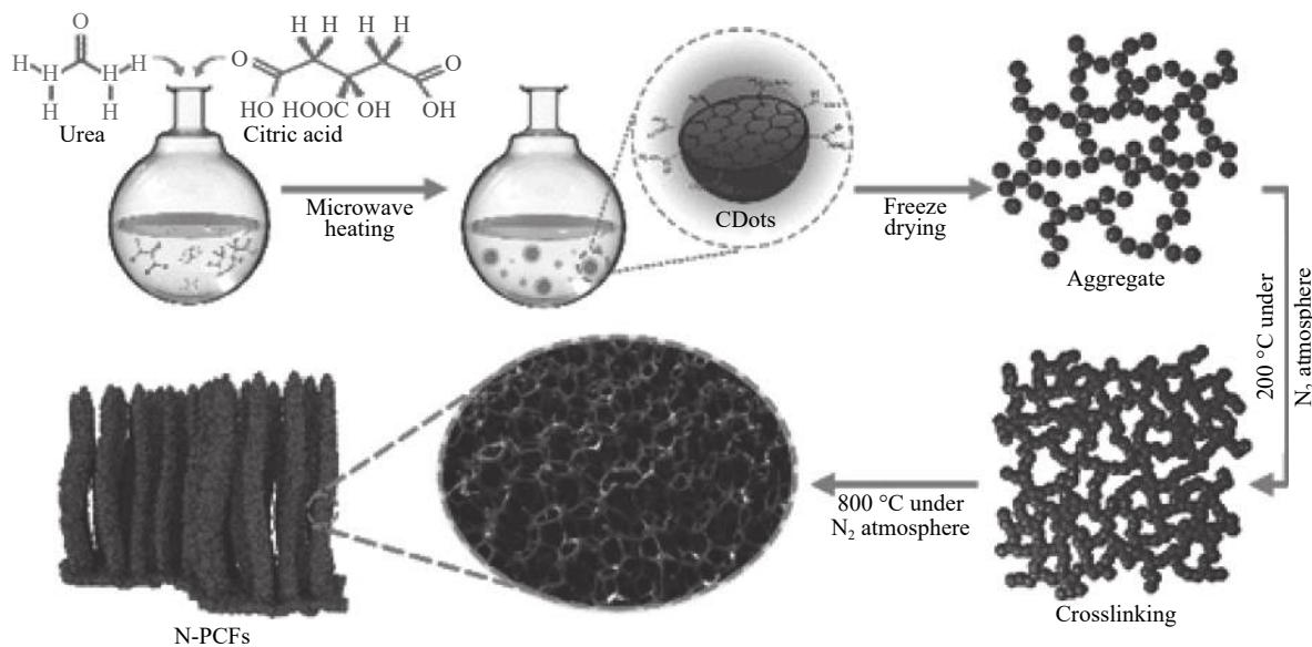
图 14 CDs 和随后合成的 N-PCFs 的示意图<sup>[58]</sup>Fig. 14 Schematic diagram of growth mechanism for the CDs and subsequently synthesized N-PCFs<sup>[58]</sup>
