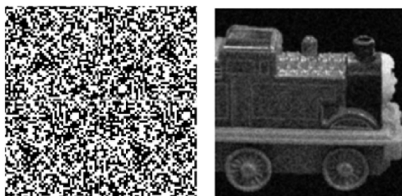
(b) 基于超分辨的 CASSI 系统恢复图和编码模板 (b) Recovery diagram and coding template of CASSI system based on super resolution
