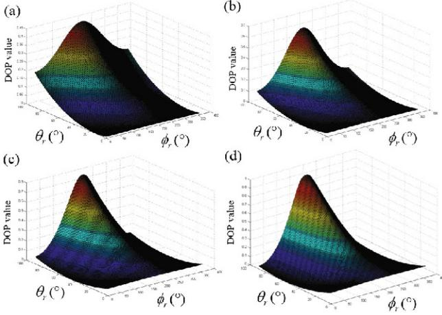
Fig. 2. (Color online) Solar panel polarization characteristics with sunlight incident at angles of (a)  $(15^\circ, 0^\circ)$ , (b)  $(30^\circ, 0^\circ)$ , (c)  $(45^\circ, 0^\circ)$ , and (d)  $(60^\circ, 0^\circ)$ .
