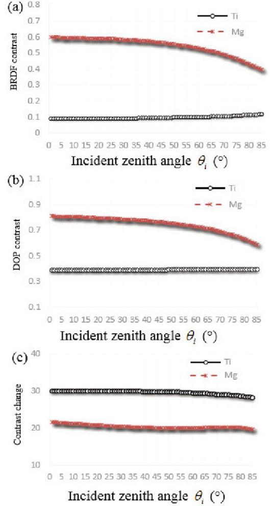
Fig. 5. (Color online) Analysis results for the (a) BRDF contrast, (b) DOP contrast, and (c) contrast change as functions of the incident zenith angle.
