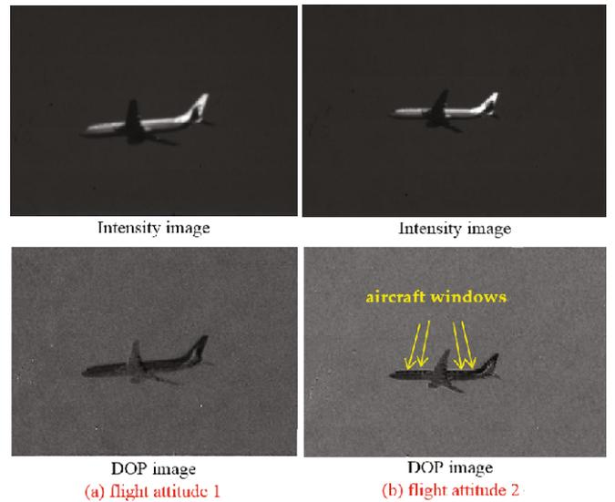
Fig. 10. (Color online) Comparison of the outfield image effects under flight attitudes (a) 1 and (b) 2.
