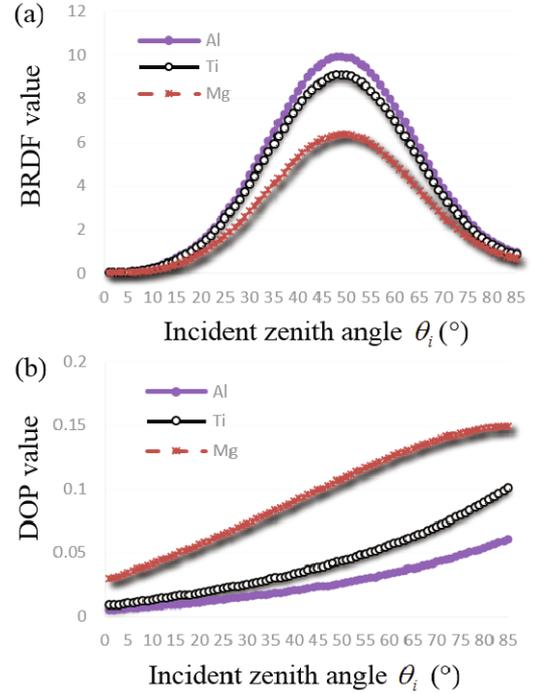
Fig. 4. (Color online) (a) BRDF and (b) DOP analyses results for different materials as functions of the incident zenith angle.
