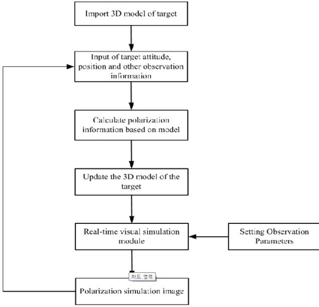
Fig. 6. Flow chart for the modeling and analysis of the space target polarization characteristics.
