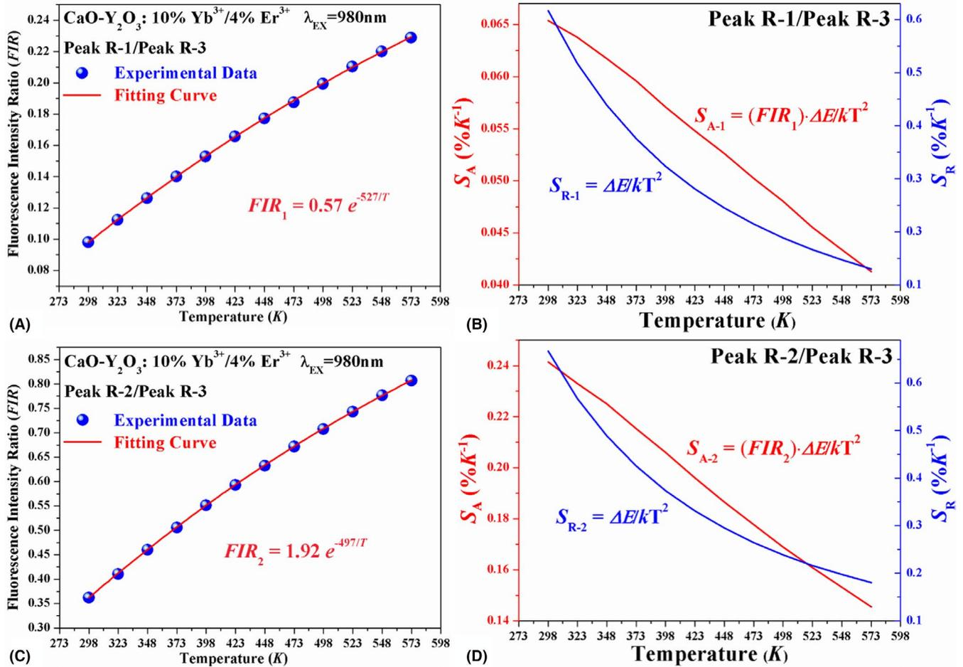
**FIGURE 5** Temperature dependence of (A)  $FIR_1$  between Peak R-1 and Peak R-3, (B)  $S_{A-1}$  and  $S_{R-1}$ , (C)  $FIR_2$  between Peak R-2 and Peak R-3 and (D)  $S_{A-2}$  and  $S_{R-2}$  in  $CaO-Y_2O_3: 10\% Yb^{3+}/4\% Er^{3+}$
