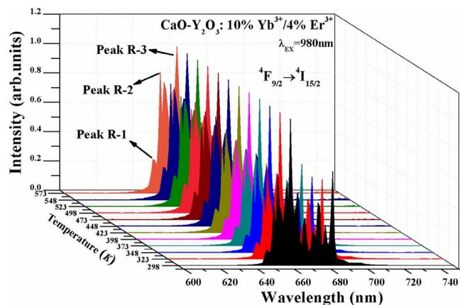
**FIGURE 4** Temperature dependence of UC spectra in CaO-Y<sub>2</sub>O<sub>3</sub>: 10% Yb<sup>3+</sup>/4% Er<sup>3+</sup> excited by 980 nm wavelength with low excitation power. The UC intensities of Peak R-3 are normalized
