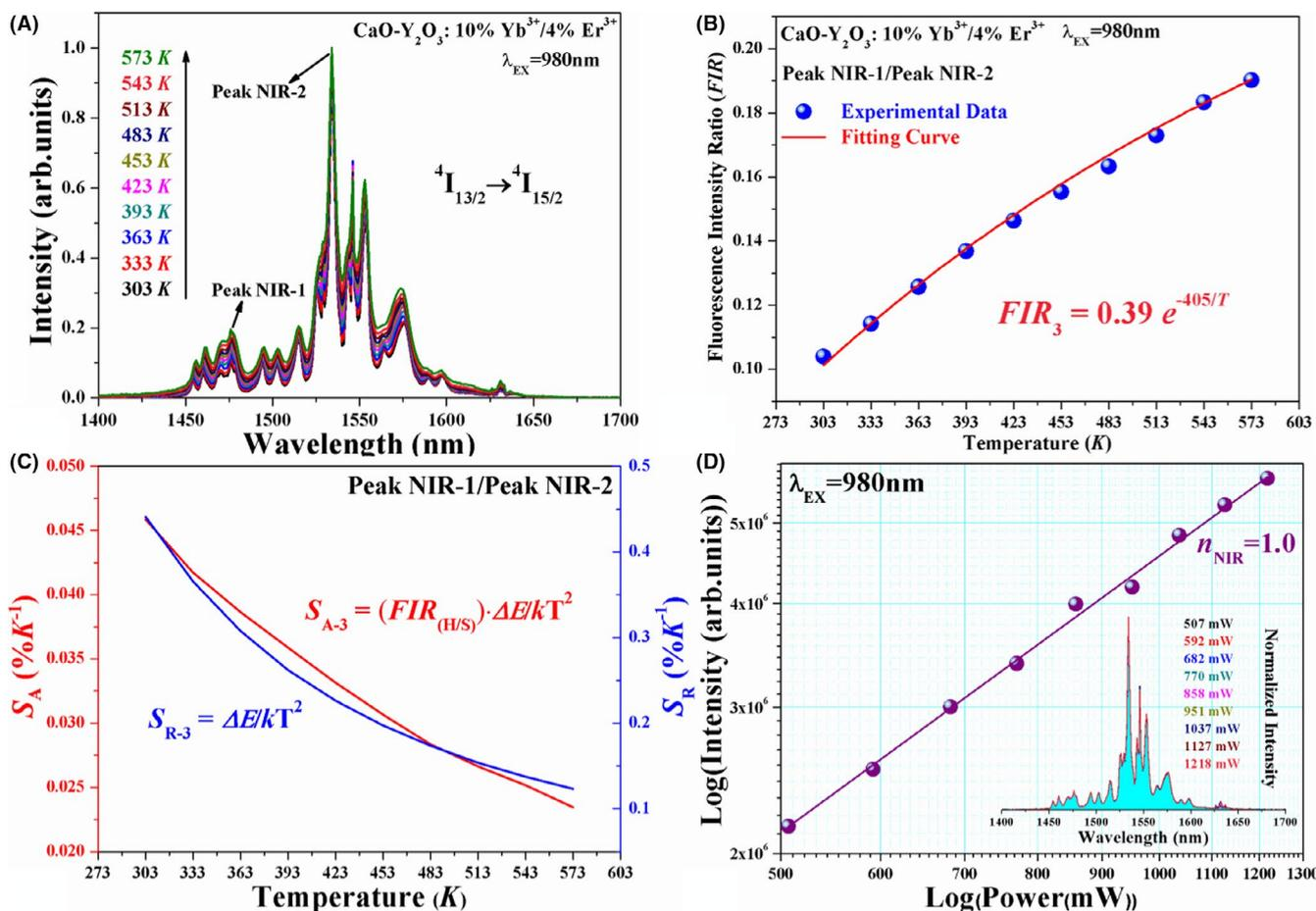
**FIGURE 8** Temperature dependence of (A)  ${}^4I_{13/2} \rightarrow {}^4I_{15/2}$  transition, (B)  $FIR_3$  between Peak NIR-1 and Peak NIR-2 and (C) the corresponding  $S_{A-3}$  and  $S_{R-3}$ . (D) Double logarithmic relationship of  ${}^4I_{13/2} \rightarrow {}^4I_{15/2}$  transition versus excitation power. Inset, the corresponding NIR spectra with normalized intensity excited by various pump power
