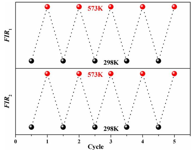
**FIGURE 6** The repeatability study in the temperature cycling between 298 and 573 K
