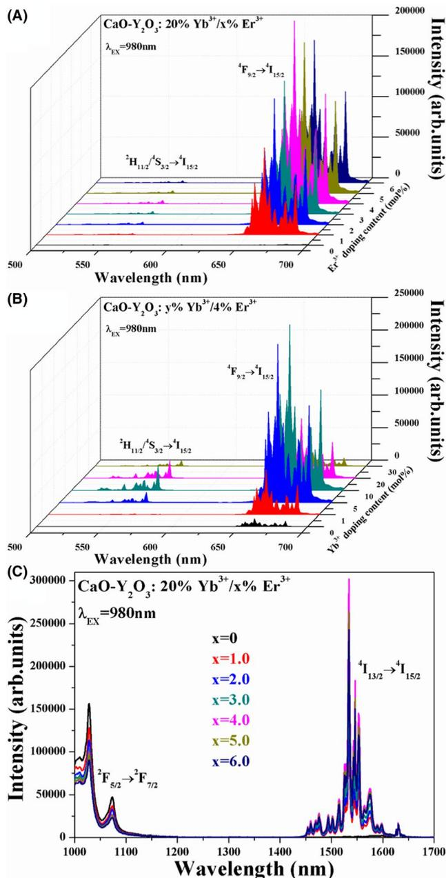
**FIGURE 2** The UC spectra of (A)  $CaO-Y_2O_3: 20\% Yb^{3+}/x\% Er^{3+}$  ( $x = 0, 1, 2, 3, 4, 5, 6$ ) and (B)  $CaO-Y_2O_3: y\% Yb^{3+}/4\% Er^{3+}$  ( $y = 0, 1, 5, 10, 20, 30$ ). (C) The NIR spectra of  $CaO-Y_2O_3: 20\% Yb^{3+}/x\% Er^{3+}$
