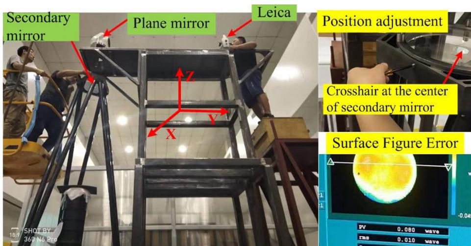
Fig. 14. Precise adjustment of secondary mirror.
