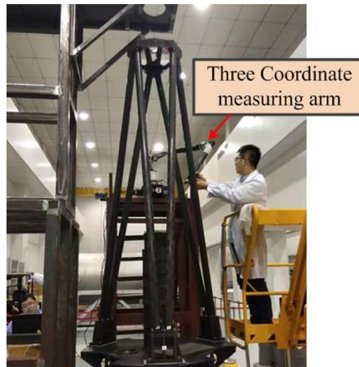
Fig. 16. Stability test in optical axis direction.
