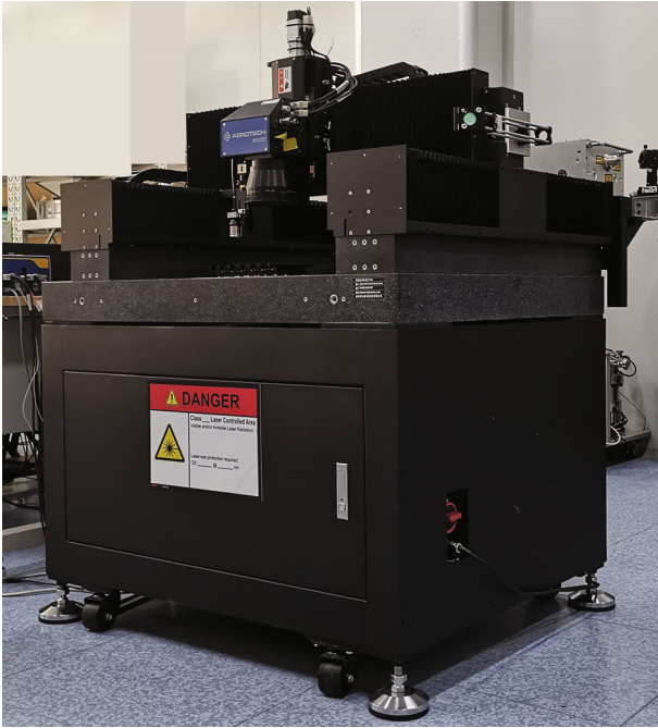
Fig. 4. Gantry for the flatness measurement.
