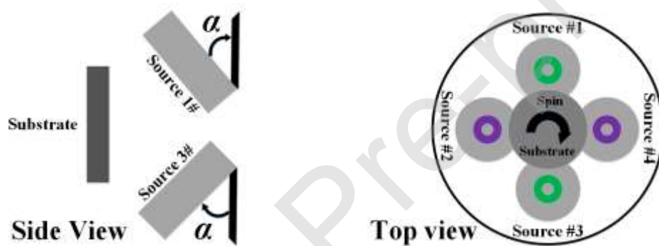
Figure 3 Sputtering sources configured in con-focal tilt mode in our deposition chamber.
